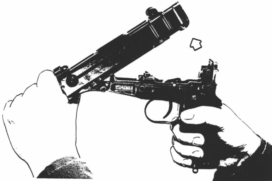
Fig. 7 - Turning of bolt guide
