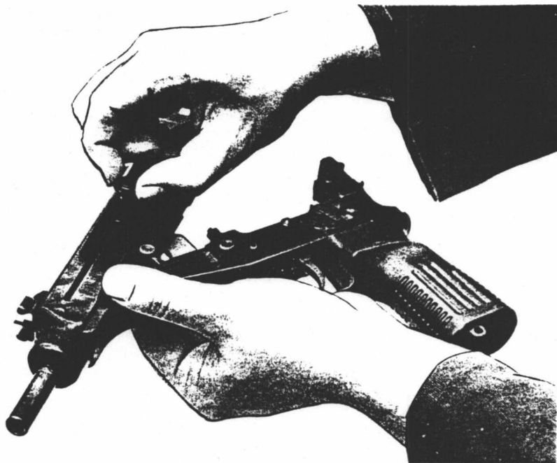
Fig. 9 - Separation of bolt cocking parts
