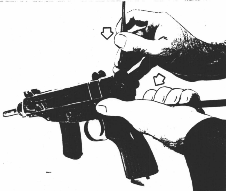
Fig. 4 - Disengagement of stock catch
