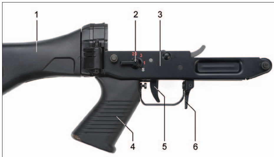
Figure 16: Trigger assembly and butt stock from right
