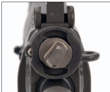
Figure 38: Gas valve in position II
