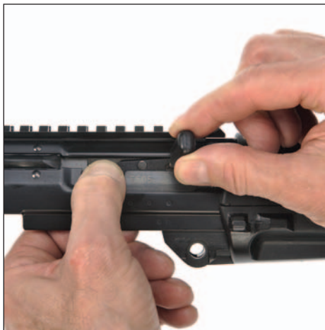
Figure 48: Remove charging handle
