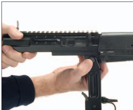
Figure 47: Remove trigger assembly
