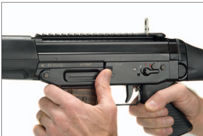
Figure 27: Push the bolt catch up
