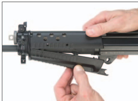
Figure 52: Lift off lower handguard
