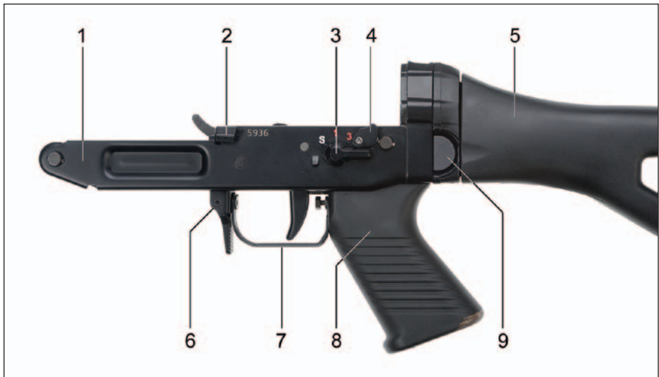
Figure 17: Trigger assembly and butt stock from left
