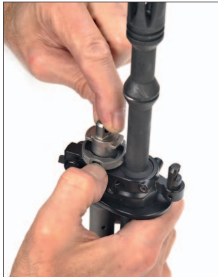
Figure 53: Remove gas valve
