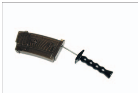
Figure 56: Stripping the magazine
