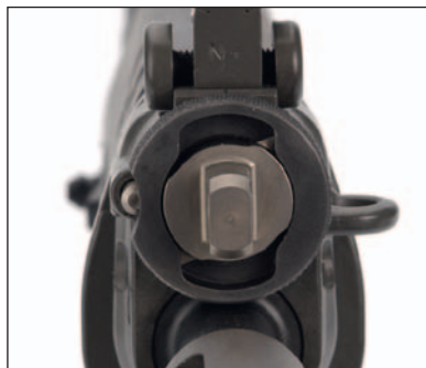
Figure 37: Gas valve in position I
