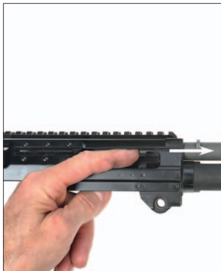
Figure 54: Remove gas piston
