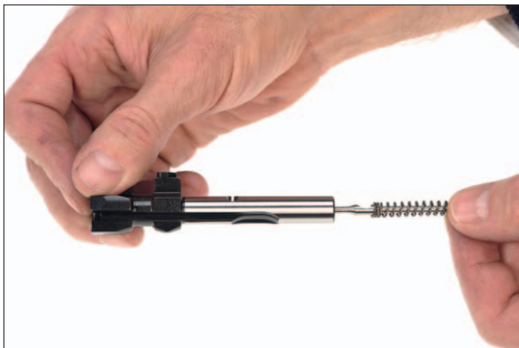
Figure 61: Install firing pin
