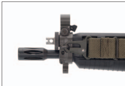
Figure 43: Sling hooked to front sight mount
