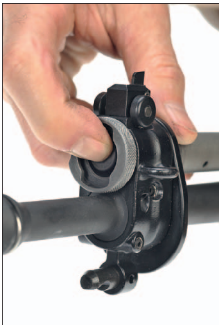
Figure 62: Check gas piston position
