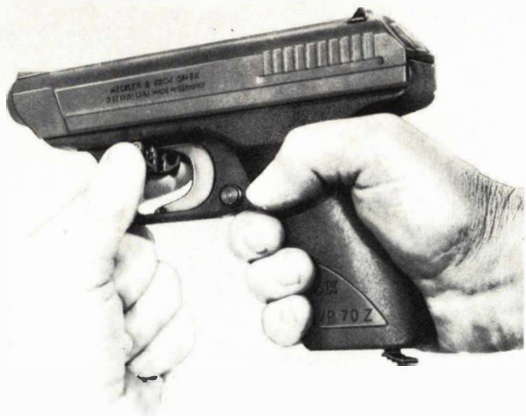
Fig. 6: Pull retaining catch downward
